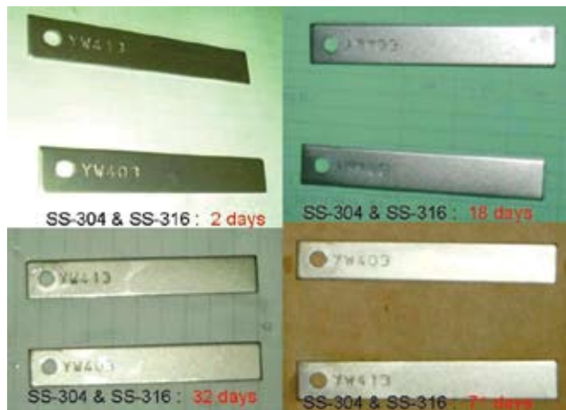
图3: 采用Amox处理后, 侵蚀试验块没有任何侵蚀迹象 Figure 3: Corrosion coupons show no evidence of corrosion after Amox treatment
