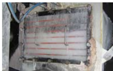
在使用AMOX的17天之后，上方喷浆成形器窥镜的视野还是很清晰的 The sight glass of top former was kept clean even after running for 17 days with Amox
