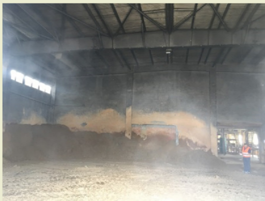
Figure 7. Odor neutralization via spray in effluent dry sludge collection room in paper mill. Odorous gas concentration reduced by 50-60% after the application
