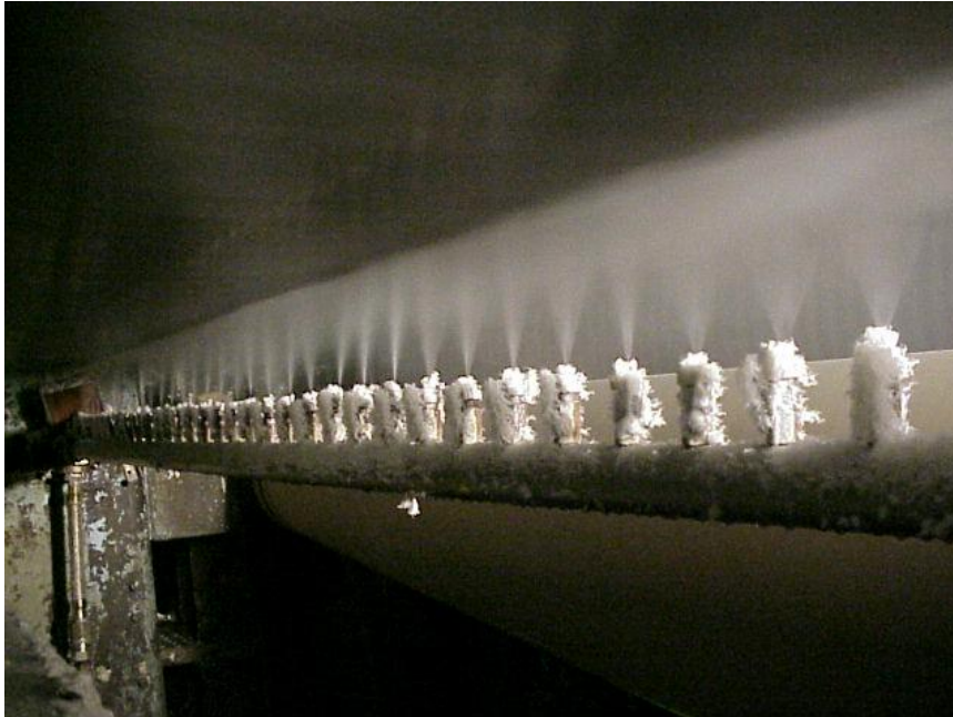
A good spray pattern is essential for an even coating to produce an even fine crepe structure.
