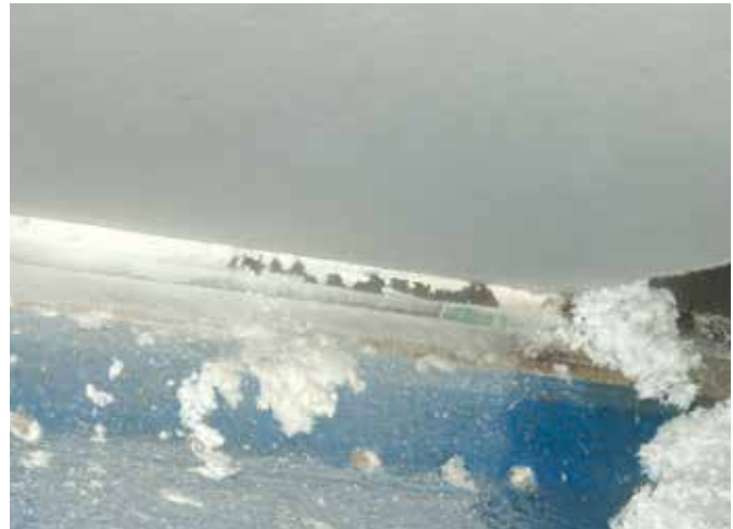
Good sheet breakdown at the doctor blade increases the fibres in the "Z" direction and improves the hand feel.
