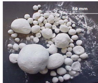
Pic4- Nodules larger than 25 mm have a dark, uncalcined grey core, surrounded by a white calcined shell (3)
